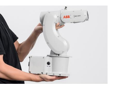
A small robot with a big performance designed to meet the trend towards the manufacture of miniaturized electronics and wearable devices. With the highest payload of 1.5kg, class-leading precision 0.01mm, and 30% smaller size, the IRB 1010 allows for the highest productivity and high-quality manufacturing.
